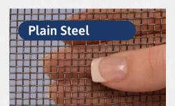
Fireplace screen mesh materials include plain steel, otherwise known as low-carbon steel. While nononsense plain steel is not as resistant to corrosion as stainless, it's both affordable and tough. Plain steel can be painted or coated for attractiveness.
