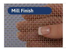
Mill finish refers to the surface finish of mesh after it is manufactured. The texture is usually rough, but some mill finished mesh is also polished, smooth, and uniform.
